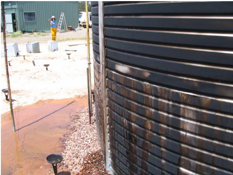
Figure 39 Experiment 24 - pre-radiation and flame immersion on Bladder tank
