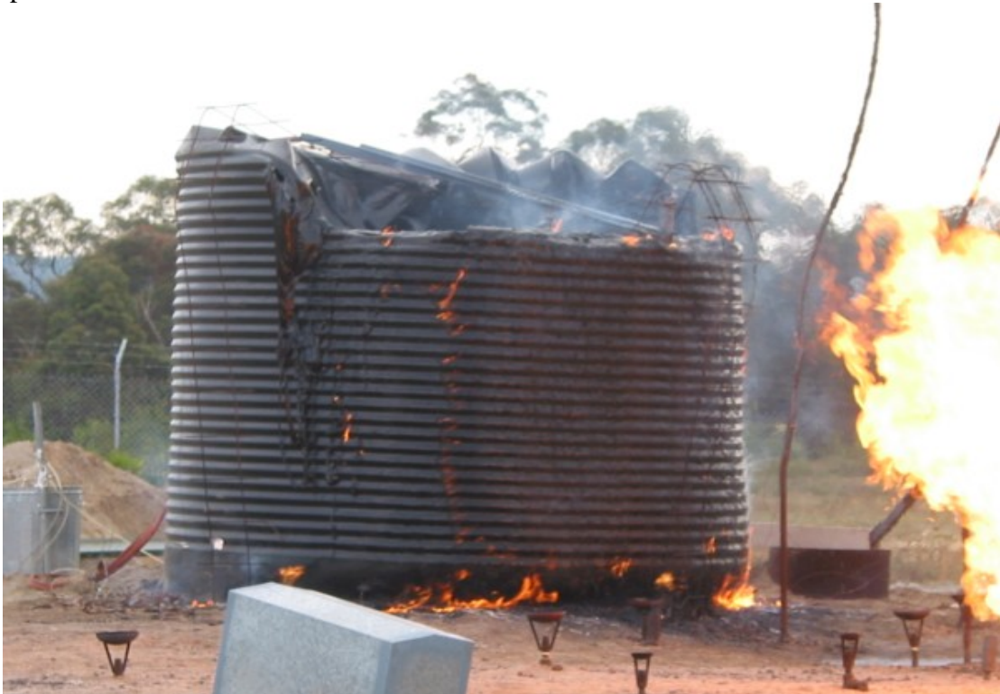
Figure C50 Tank 8 ignition and failure above waterline as a result of litter ignition and pre-radiation and flame exposure.
