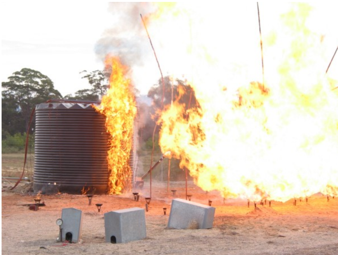
Figure C44 Tank 8 ignition as a result of litter ignition and pre-radiation exposure.
