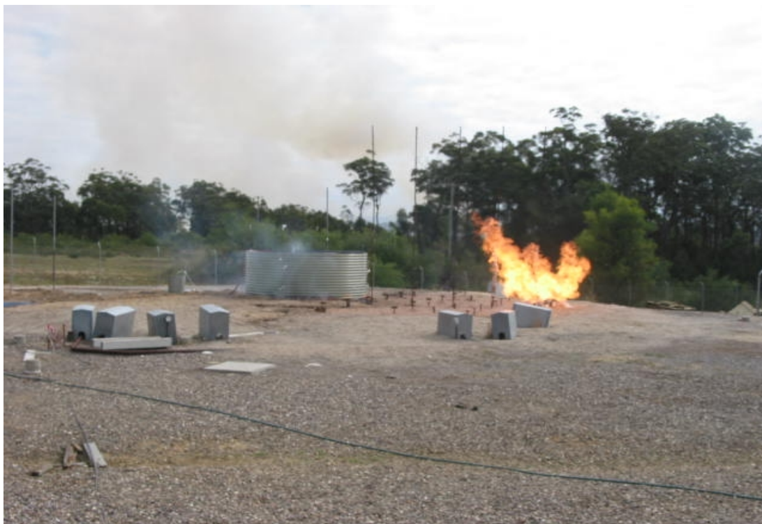
Figure C1 Tank one, metal tank with plastic coating, Pre Radiation exposure.
