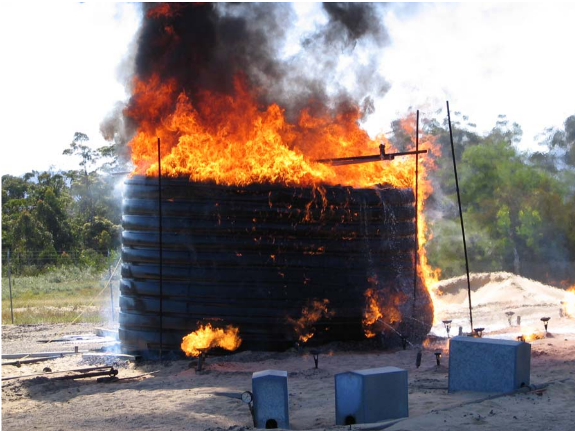
Figure 43 Experiment 26 - Pre-radiation and flame exposure on used polyethylene tank
