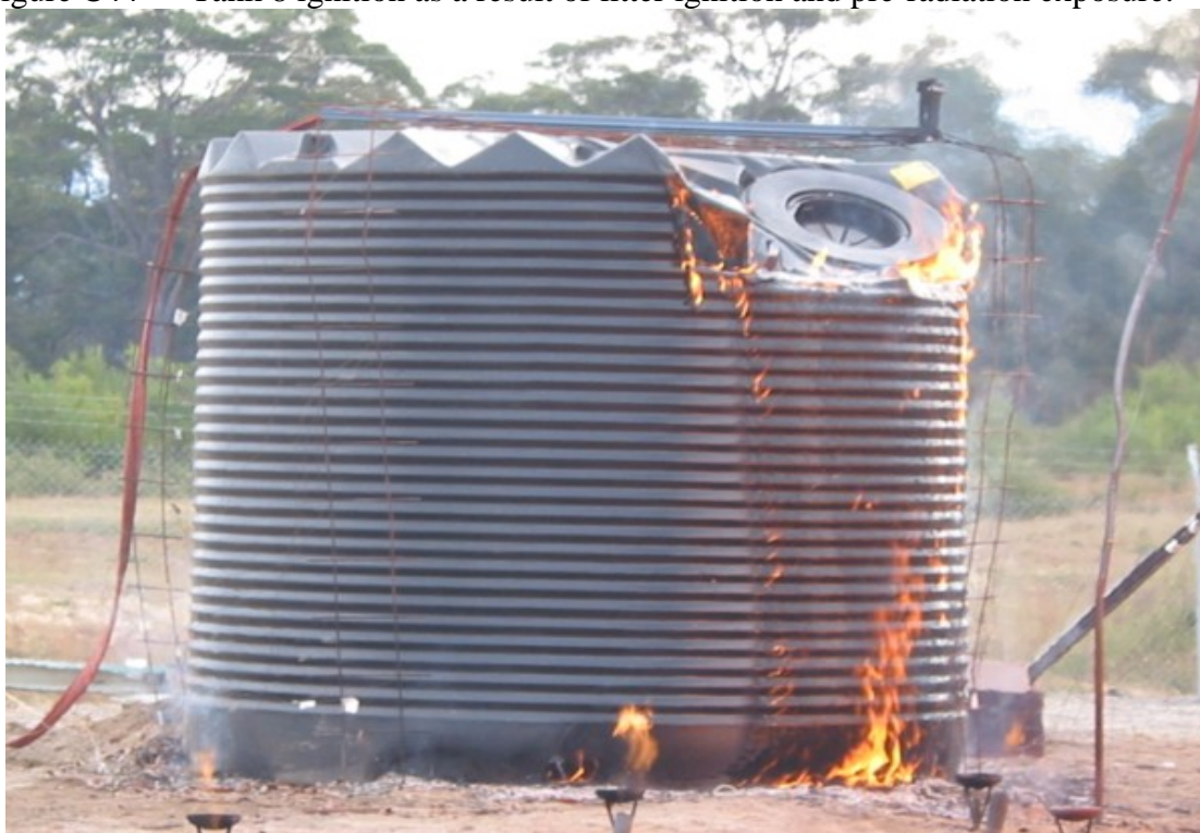
Figure C45 Tank 8 ignition as a result of litter ignition and pre-radiation exposure. Flowing water from the collapsing upper portion of the tank assisting extinguishing flames.
