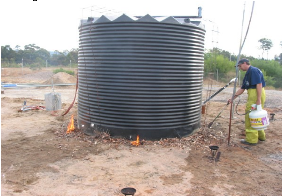
Figure C41 Tank 8 litter ignition .
