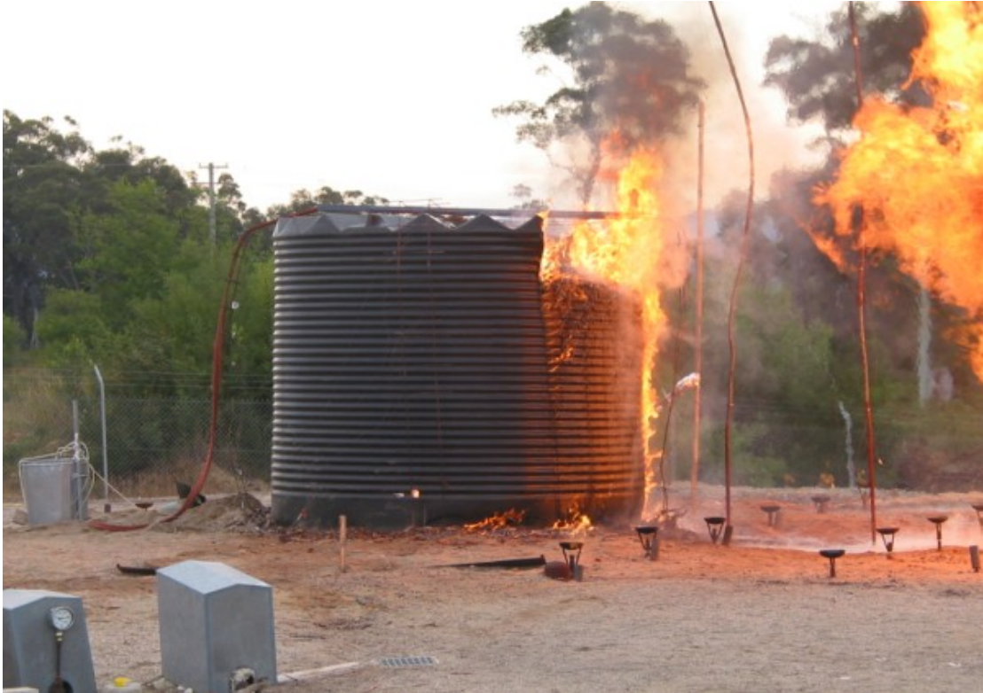
Figure C47 Tank 8 ignition as a result of litter ignition and pre-radiation and flame exposure.
