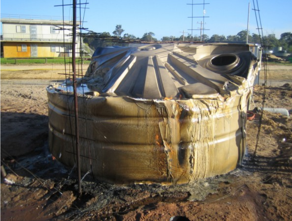
Figure 11 Experiment 5 - Pre-radiation exposure on polyethylene tank (note water stream from the base of the tank)
