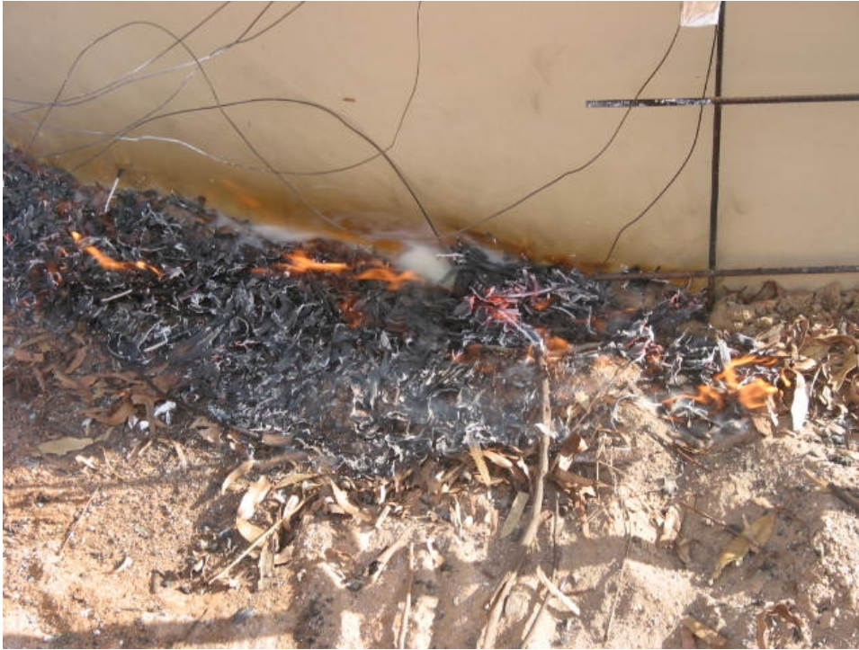
Figure 8 Experiment 4 - Leaf litter exposure on polyethylene tank
