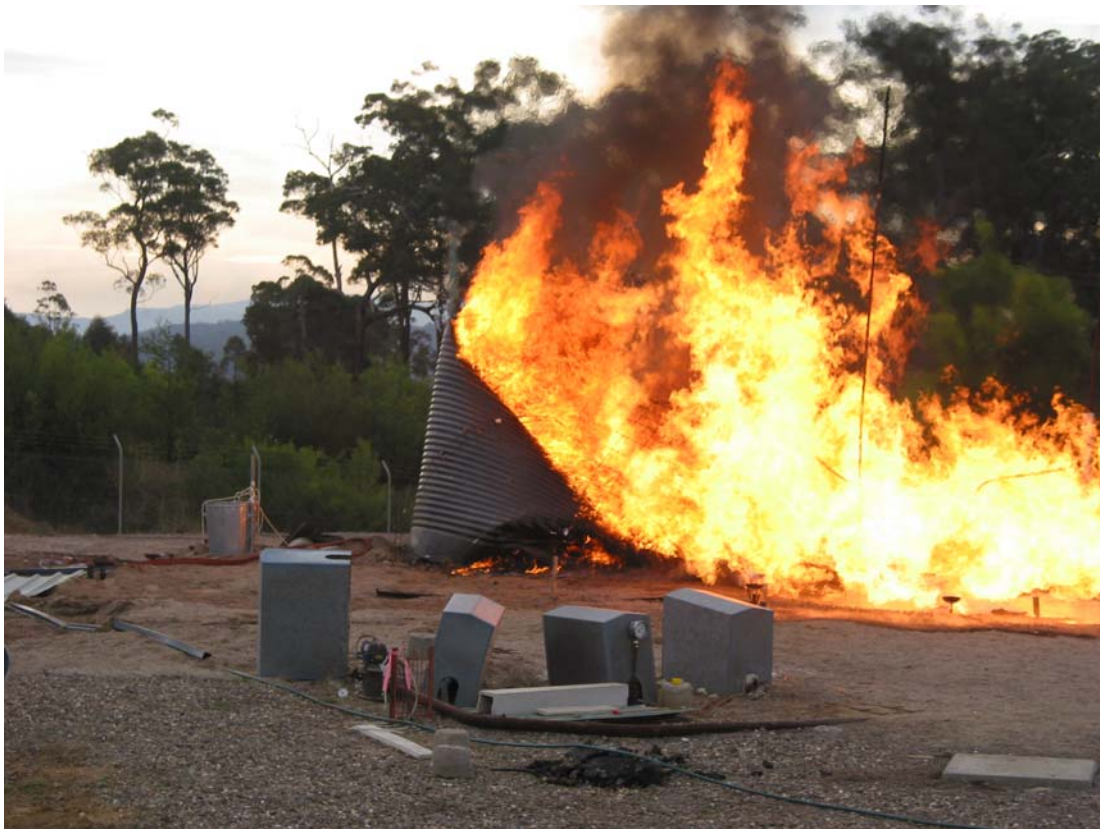
Figure C53 Tank 8 ignition and initial stages of failure due to structural fire exposure.
