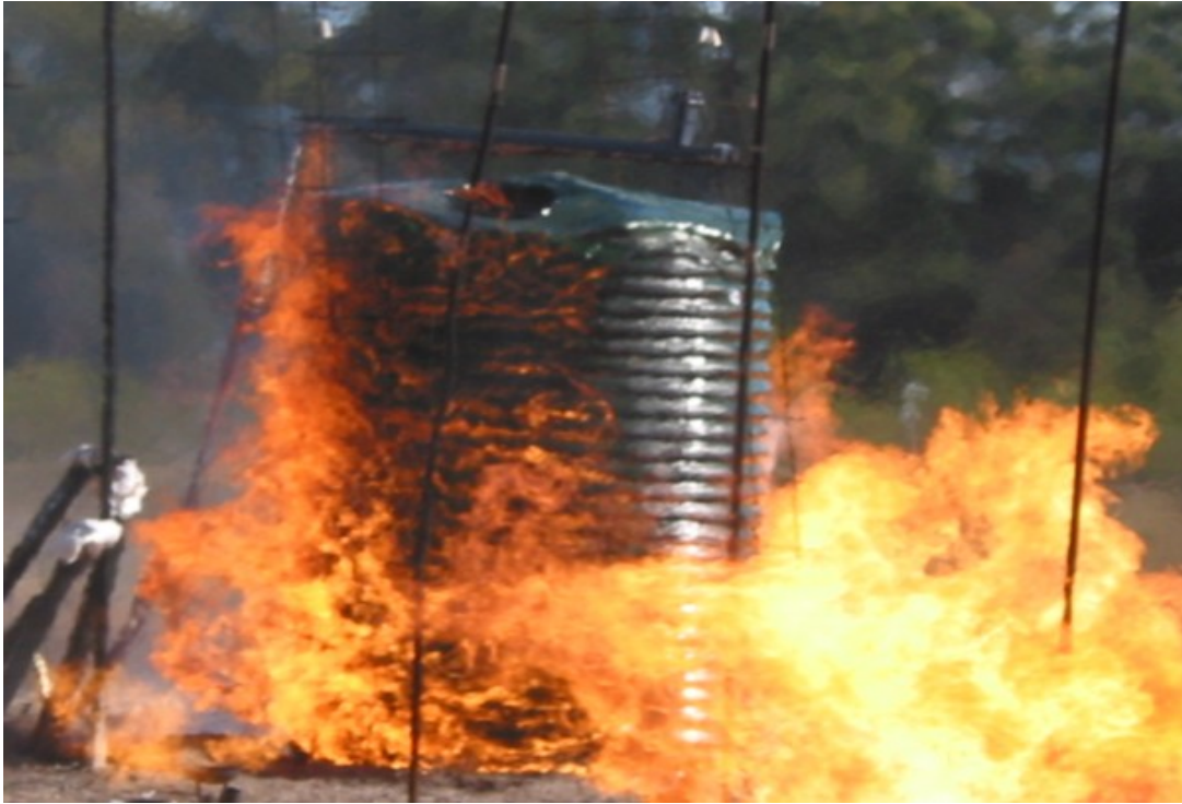
Figure C28 Tank four flame exposure.
