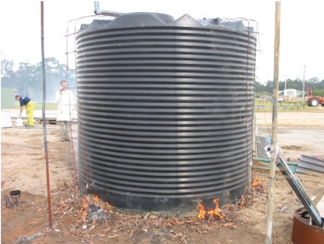
Figure C42 Tank 8 litter ignition .
