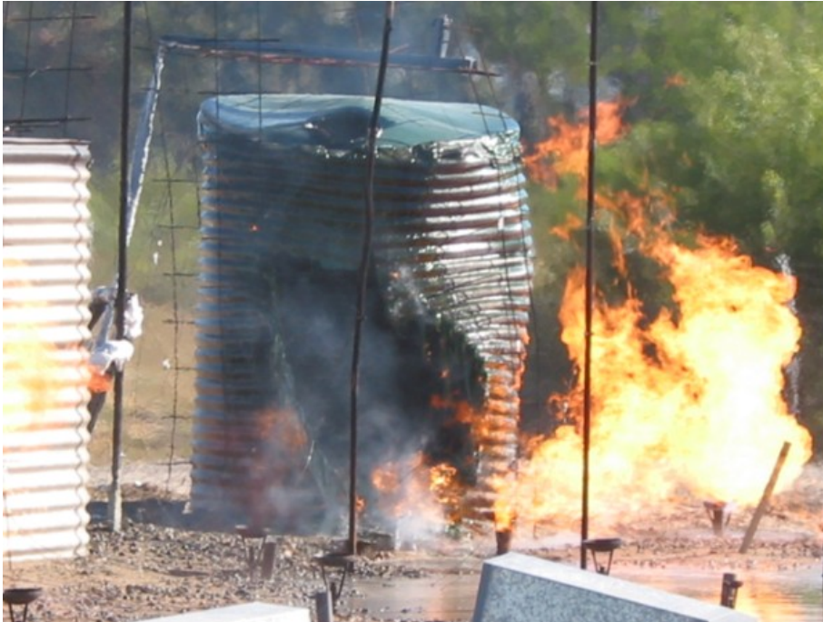
Figure 21 Experiment 14 - Structure exposure on polyethylene and metal tank
