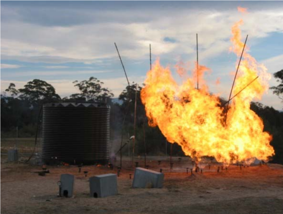
Figure 29 Experiment 19 – Radiant heat flux – Tank 8 Polyethylene black
