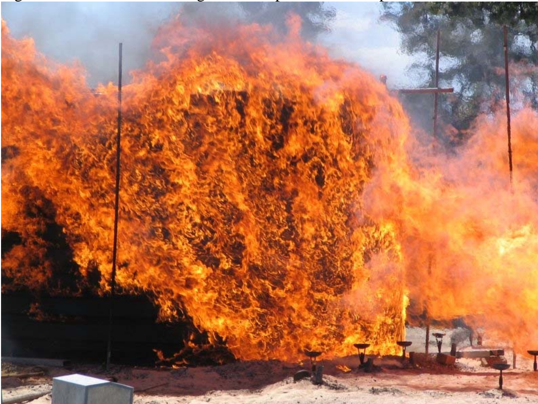
Figure C69 Ignition of tank 10 during the litter ignition and pre-radiation exposure.
