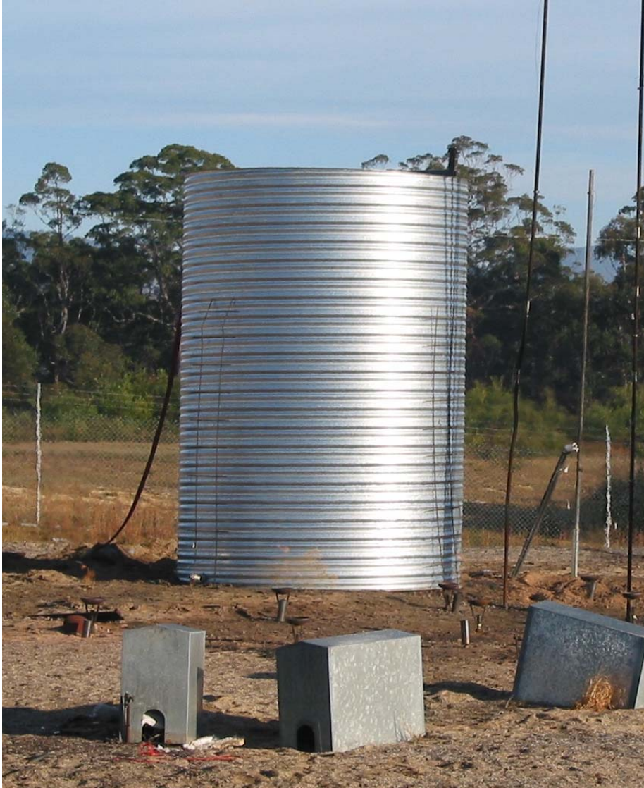
Figure 25 Experiment 16 – Radiant heat flux – Tank 7 Spiral wound metal galvanised
