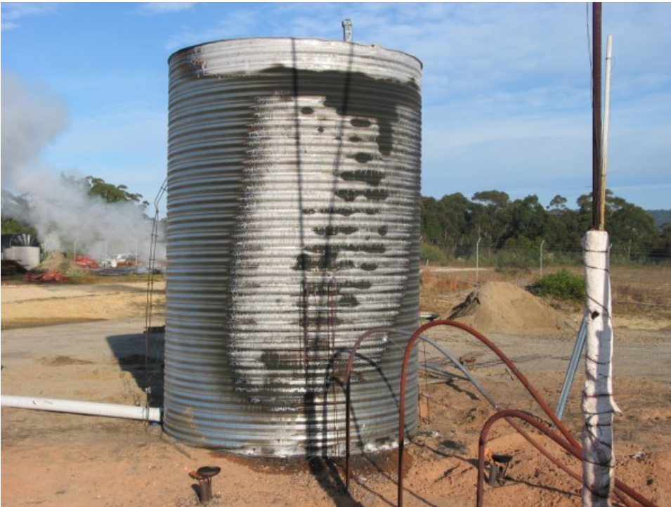
Figure 27 Experiment 17- Structure exposure on metal spiral tank
