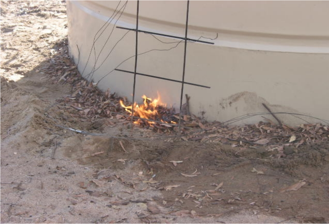
Figure C7 Tank six Litter ignition.
