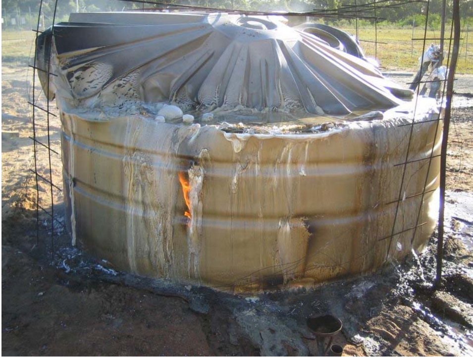
Figure 12 Experiment 6 - Structure exposure on polyethylene tank
