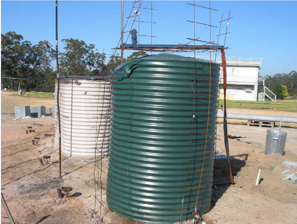
Figure 18 Experiment 12 - Pre-radiation exposure on polyethylene and metal tank
