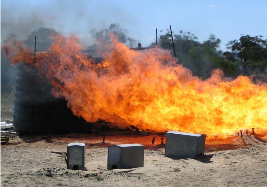
Figure C72 Tank 10 litter ignition, pre-radiation and flame exposure.
