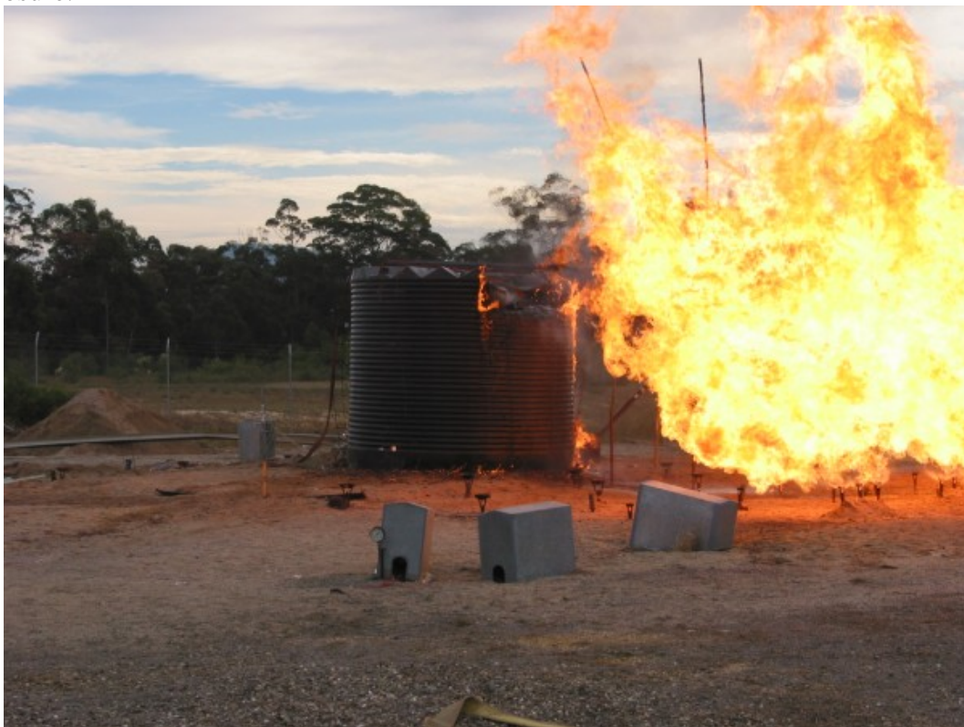
Figure C48 Tank 8 ignition as a result of litter ignition and pre-radiation and flame exposure.
