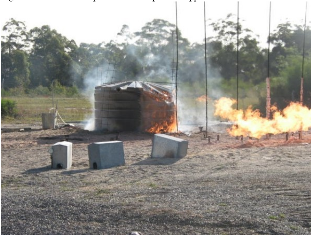
Figure C10 Tank six ignition and flaming due to pre radiation exposure.
